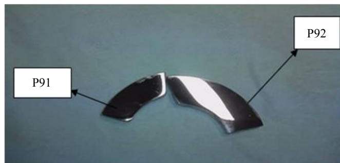
Fig. 1. The appearance of P91 and P92 samples when they are ready to test, after undergoing cutting, grinding and polishing processes
